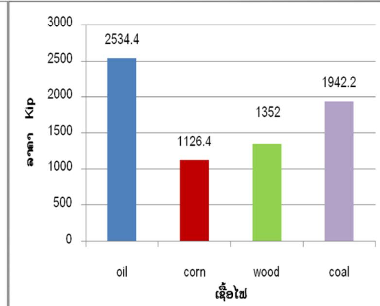
Left figure shows the results of experiment how much money should pay for fuel when used producer gas from corn cob, waste wood and charcoal integrated with diesel fuel as dual fuel and also for diesel oil alone for running diesel engine with different speed.
