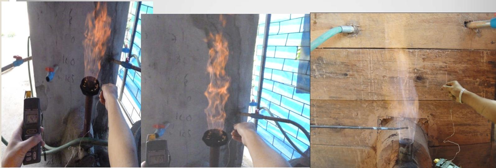
The Flame of combustion producer gas for cob corn, wood waste, and charcoal as fuels respectively.
