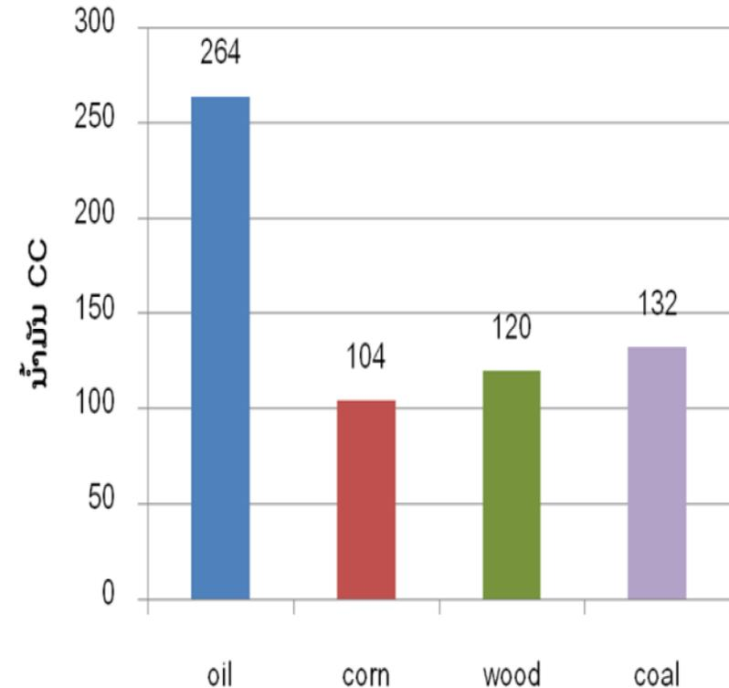
These figures show the results of experiment how many CC can save diesel oil when used producer gas from corn cob, waste wood and charcoal integrated with diesel fuel as dual fuel for running diesel engine with different speed
